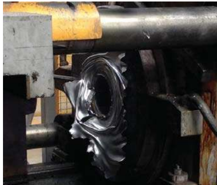
Figure 11. The flash overflow of the material without billet buckle angle in the upper die.
