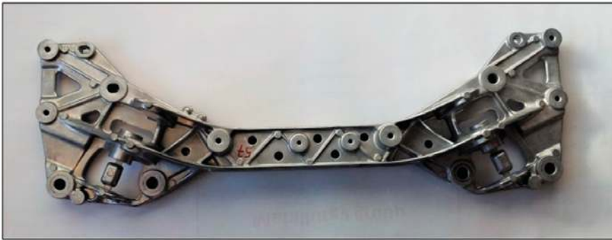
Figure 12. Hollowed aluminum high pressure die casting component.
